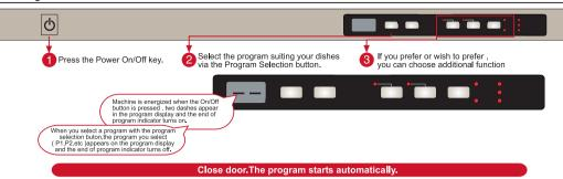
Note:If you decide not to start to machine after selecting the program, just press the on/off button. Your machine will become ready for the new program selection when you press on/off button again. You can select the new program by pressing the program selection button.
