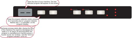
Note: When the door of the machine is opened in order to stop the washing program before it is completed first open the door slightly in order to avoid water spillage.
